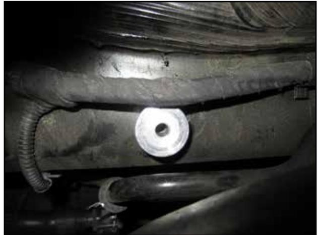
e. Set provided spacer (L) in place. Position the spacer in the indicated location.
