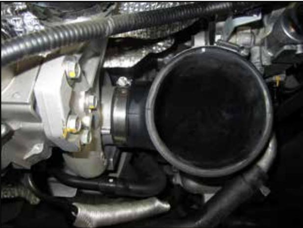
d. Install the coupler (H) onto the Turbo inlet using the provided hose clamps (G) and (I).
