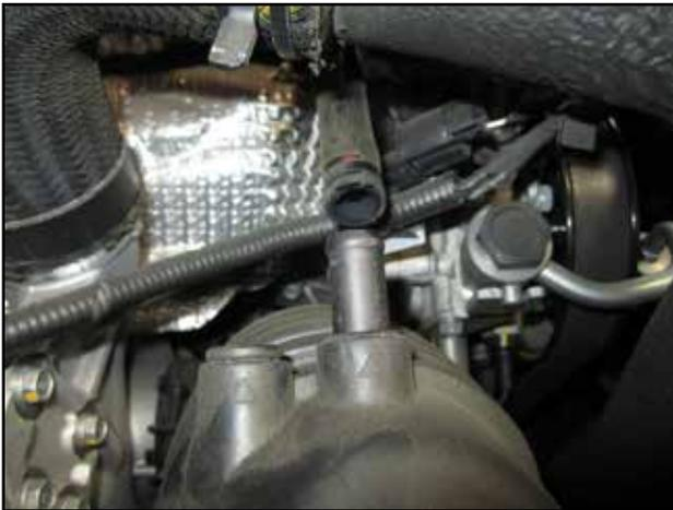
g. Release the clips on the two PCV hoses (Manual Trans) and disconnect the hoses from the intake tube. (Automatic shown)
