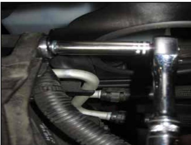
p. Now tighten the front M6 bolt installed in step n.
