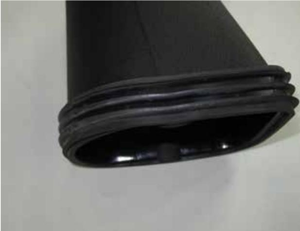
b. Install the OEM rubber gasket on the AEM scoop adapter (A)
