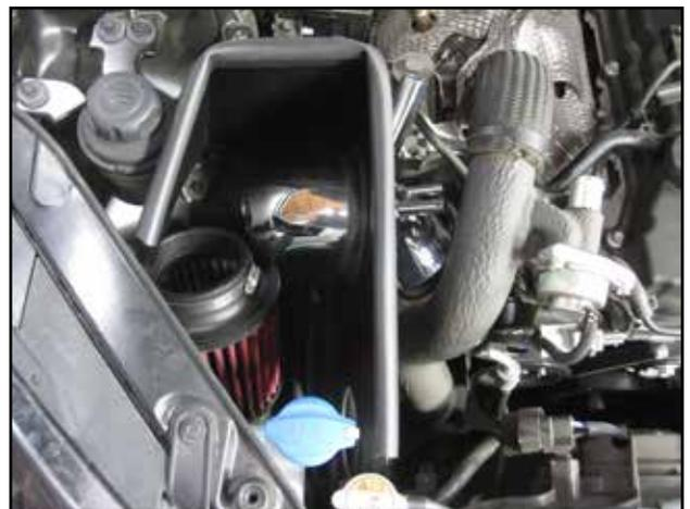
k. Set heat shield (O) and intake tube (B) in place.
