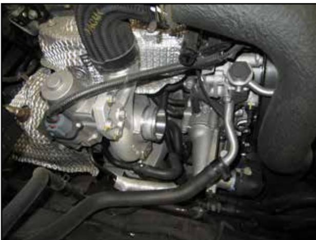
i. Remove the intake tube from the engine bay.
