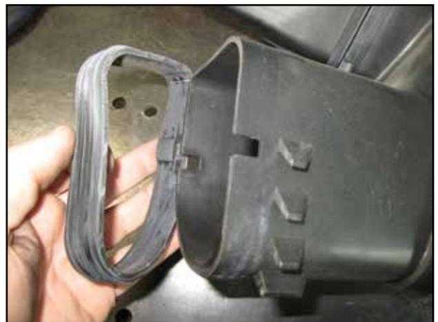
j. Remove the seal from the air box.
