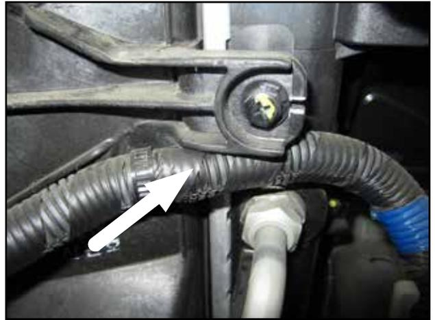
c. Remove the bolt on the fan shroud.
